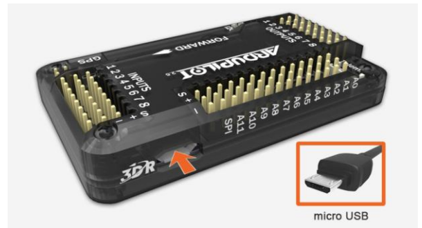
Figure 4.2: APM 2.6 micro USB port
