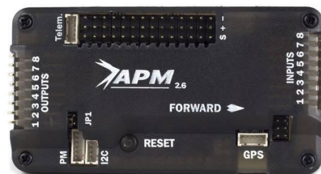
Figure 3.7: APM inside it's protective casing
