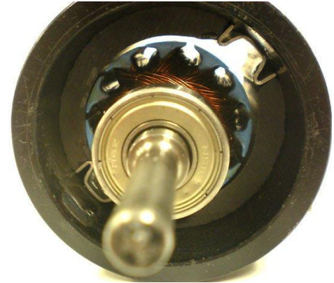
Figure 3.2: Brushed motor with windings on rotor and magnets on stator
