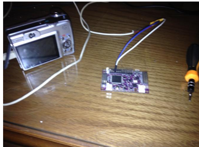
Figure 3.14: Camera connected to APM with modified cable
