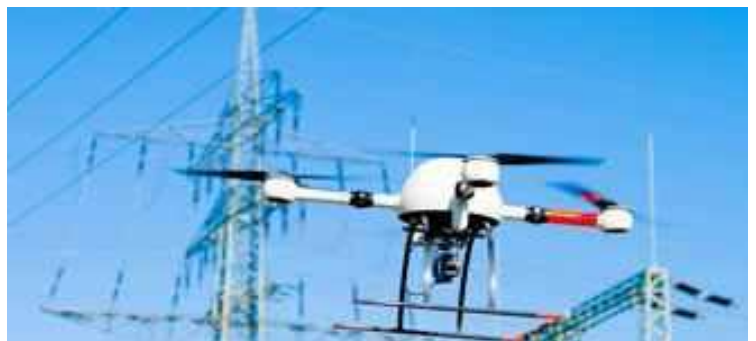
Figure 2.7: Quad used for inspection
