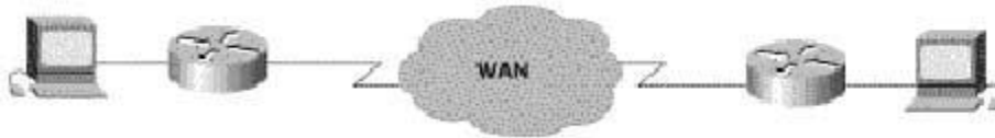
Figure 2. A Typical Point-to-Point Link Operates Through a WAN to a Remote Network
