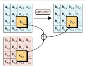
Step 4: AddRoundKey Each byte of the state is combined with a byte of the round subkey using XOR operator .
