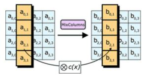
Step 3: MixColumns Each column of the state is multiplied with a fixed polynomial c(x).
