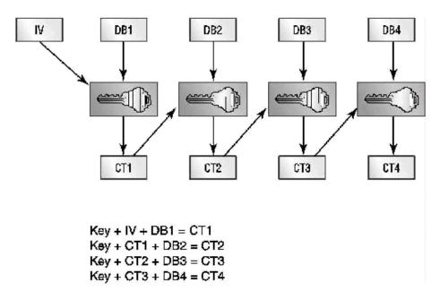
**Fig 2.15** Block cipher encryption example
