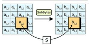
Step 1: SubBytes Each byte in the state is replaced with its entry in a fixed 8-bit lookup table, S; bij = S(aij).
