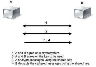
**Fig 2.13** Fig of Symmetric encryption
